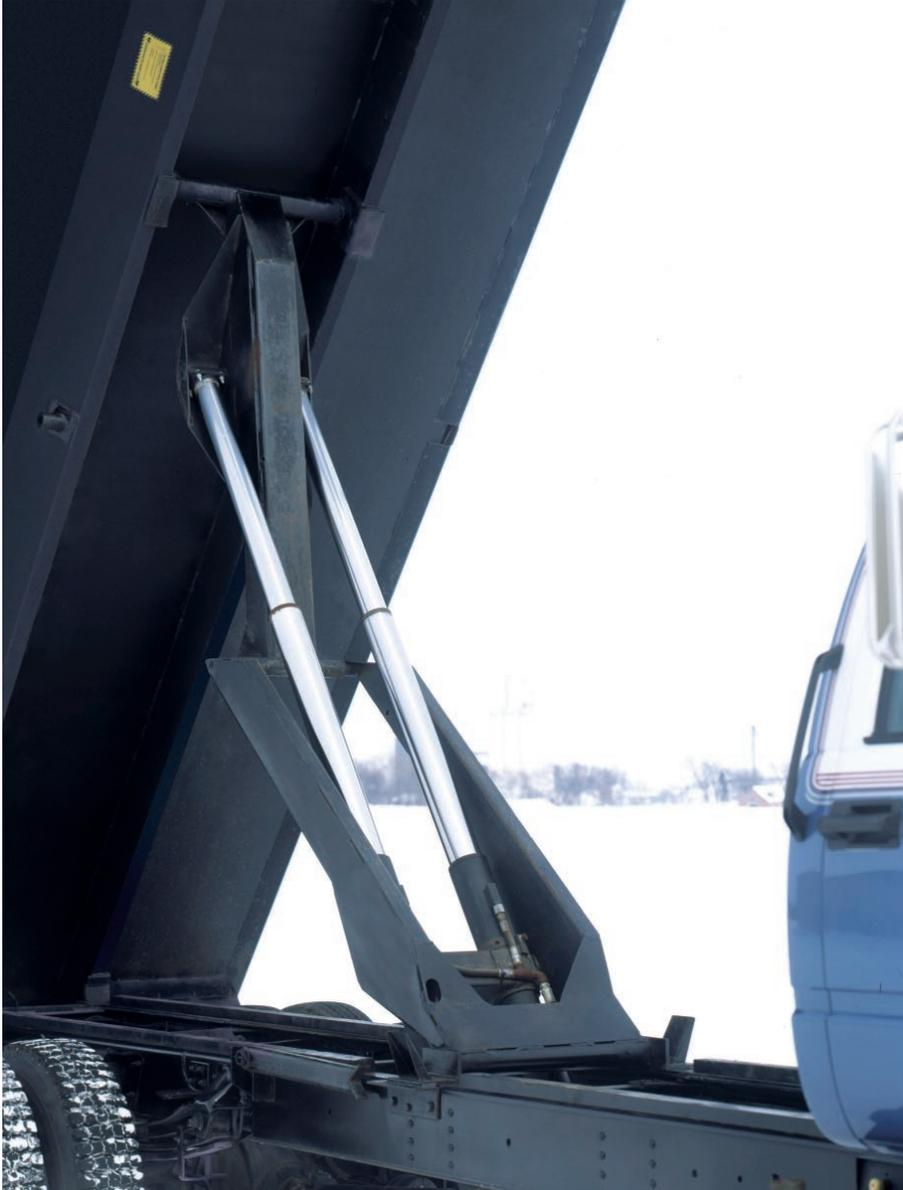
No one packs so much value into a heavy-duty hoist...with capacities from 10 to 50-ton in bodies from 10 to 28 feet long.
