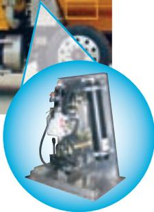
Exclusive sloped front design accommodates hydraulic cabinet, reservoir and hoist, virtually eliminating the doghouse for better cleanout.
