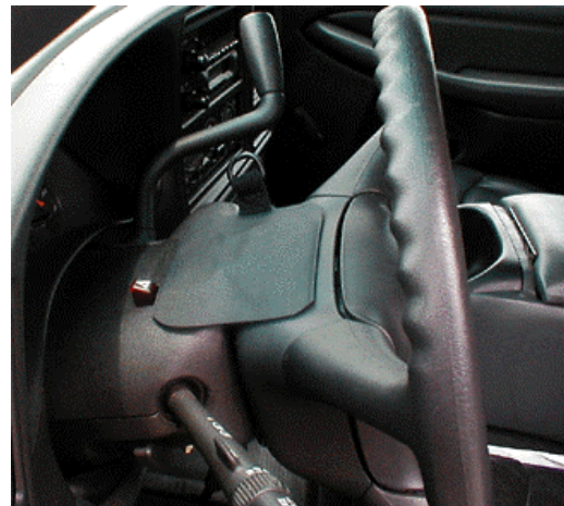
Figure 2: Steering Wheel Lock In Use
