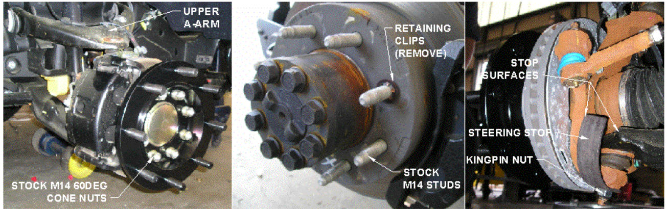
Figure 5: Wheel Adapter Details
