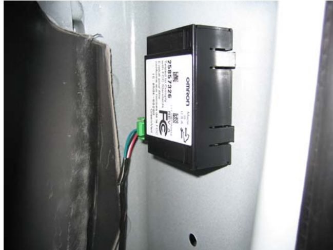
Figure 2: TPMS Receiver on B-Pillar (looking from drivers side doorway)
