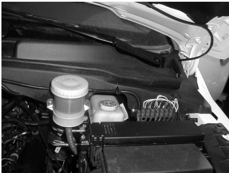
Figure 4: Typical Reservoir Installation
