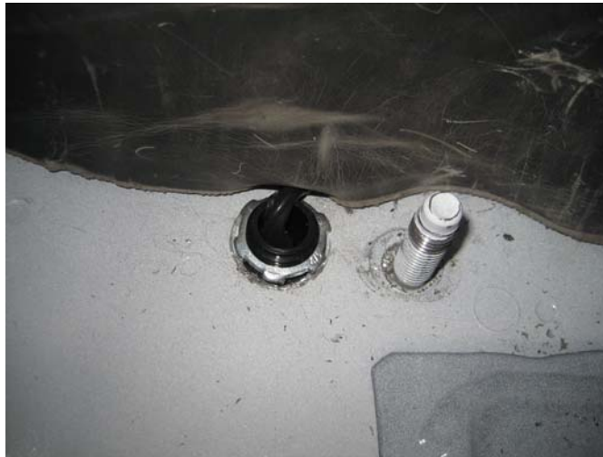
Figure 3: Floorboard Hole Location w/ Strain Relief (drivers's side to right)
