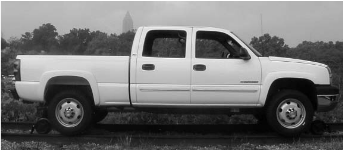
Figure 1: '03 GM/Chevy C25HD w/ RW-1013 Installed
