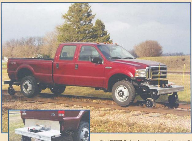
Harsco Track Technologies' HR0307 Series A HY-RAIL® Guide Wheel unit is used to adapt light duty trucks and SUVs, meeting HTT's recommended vehicle specifications, for railway applications requiring travel on the highway and on the rail.
