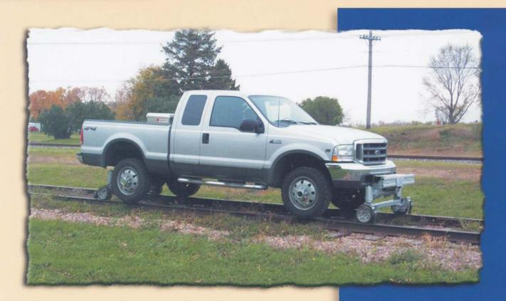
The Harsco Track Technologies **HR1500 Series B HY-RAIL®** guide wheel equipment is used to adapt light duty trucks and utility vehicles, meeting Harsco Track Technologies' recommended vehicle specifications, for highway and railway travel.
