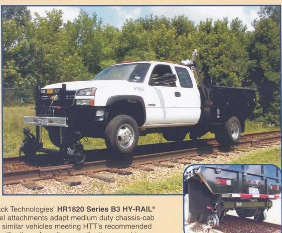
Harsco Track Technologies' HR1820 Series B3 HY-RAIL® guide wheel attachments adapt medium duty chassis-cab trucks and similar vehicles meeting HTT's recommended vehicle specifications, for railway applications requiring travel on the highway and on the rail.
