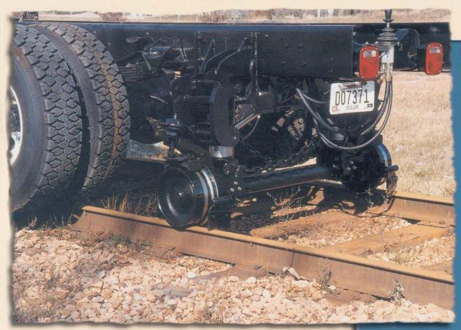
The *HR3000 Series B HY-RAIL®* guide wheel attachment is used to adapt medium-duty, chassis-cab trucks, meeting Harsco Track Technologies' recommended vehicle specifications, for highway/railway applications where a vertically-actuating rear unit is desired. This unit is ideal for applications where other equipment must also be mounted on the rear of the vehicle.
