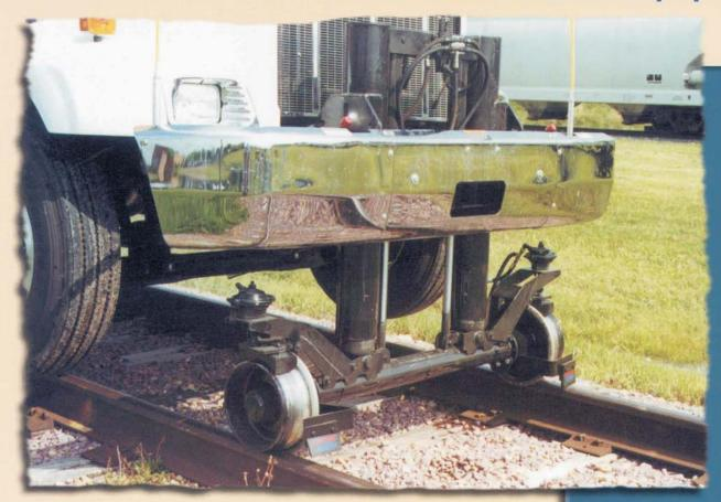
The *HR3000 Series V HY-RAIL®* guide wheel attachment is used to adapt medium-duty, chassis-cab trucks, meeting Harsco Track Technologies' recommended vehicle specifications, for highway/railway applications where a vertically-actuating front unit is desired. This unit is ideal for applications where it is necessary to minimize front unit overhang.
