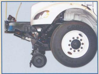
The HR3000 Series C2 HY-RAIL® guide wheel attachment is used to adapt medium-duty, chassis-cab trucks, meeting Harsco Track Technologies' recommended vehicle specifications, for highway/railway applications.
