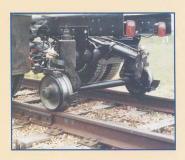
Like all HY-RAIL® guide wheel units, HR4000 Series A units are manufactured with proven HTT quality methods such as non-destructive evaluation of critical parts using x-ray and/or ultrasonic methods to assure relieable service.
