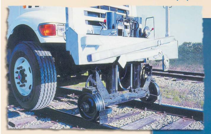
The *HR4000 Series V HY-RAIL®* guide wheel attachment is used to adapt heavy-duty, chassis-cab trucks, meeting Harsco Track Technologies' recommended vehicle specifications, for highway/railway applications where a vertically-actuating front unit is desired. This unit is ideal for applications where it is necessary to minimize front unit overhang.
