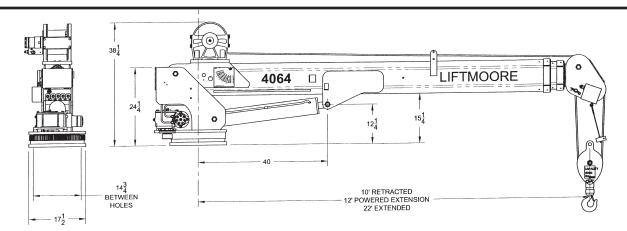
**CAPACITY:** Moment rating of 40,000 ft.-lbs. with lift capacities as follows:
